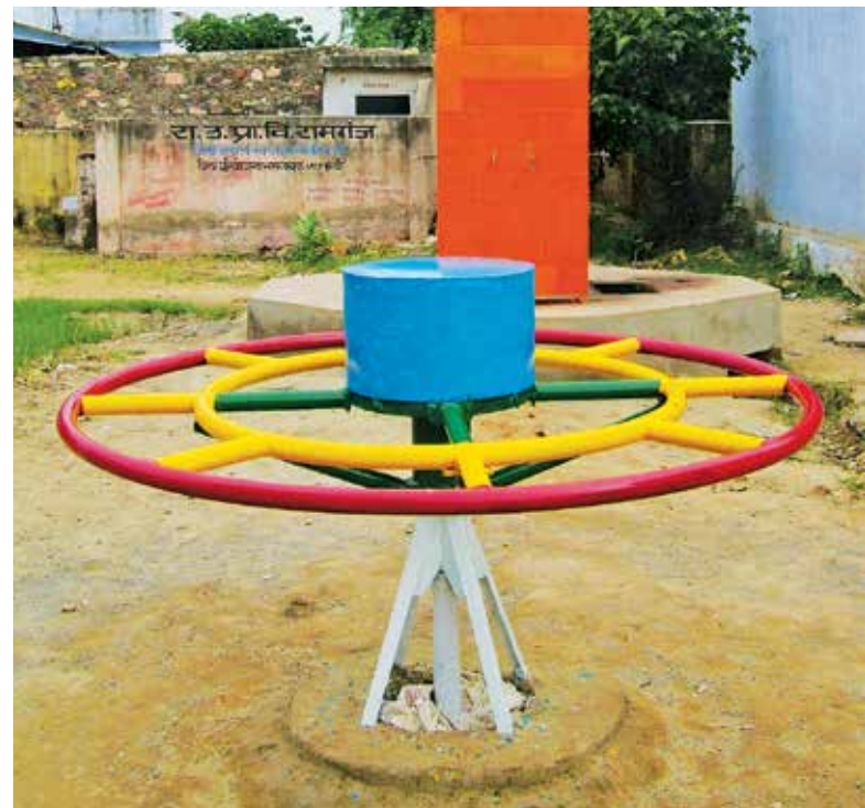
Merry go round pump: A technology that can ensure running water in schools
